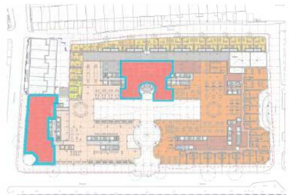
First Floor Plan - Total A1 & A3 (GEA excluding cores) : 1,395 m 2
